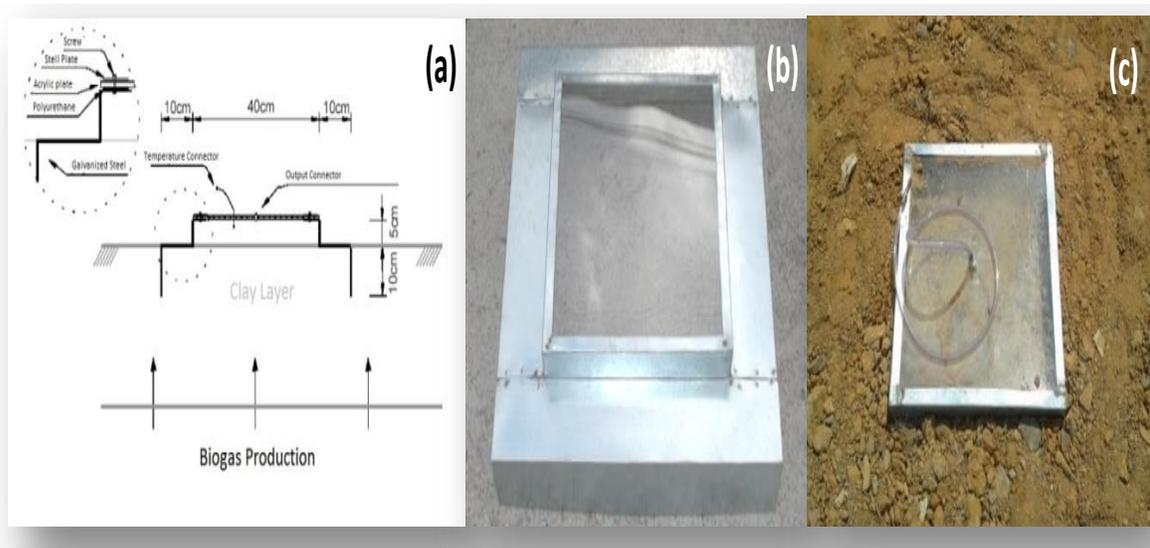
Figure 2a. Static flow plate design and settling scheme of the plate; (b) Static flow plate ready; (c) Static flow plate installed. Source: Adapted from Maciel and Juca, 2011.
