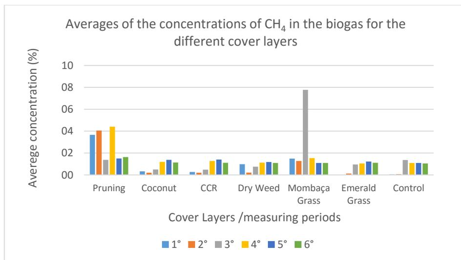
**Figure 3.** Averages of the concentrations of CH<sub>4</sub> in the biogas for the different cover layers, in the six measuring periods in 2014.
